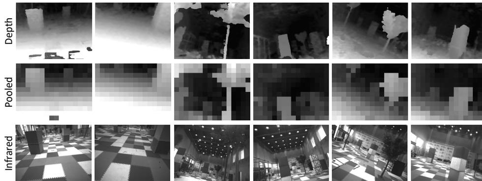
**Supplementary Fig. 4:** Depth image sequence during a sample flight, along with the pooled depth images and infrared grayscale images. See Supplementary Video 8 for the full sequence.
